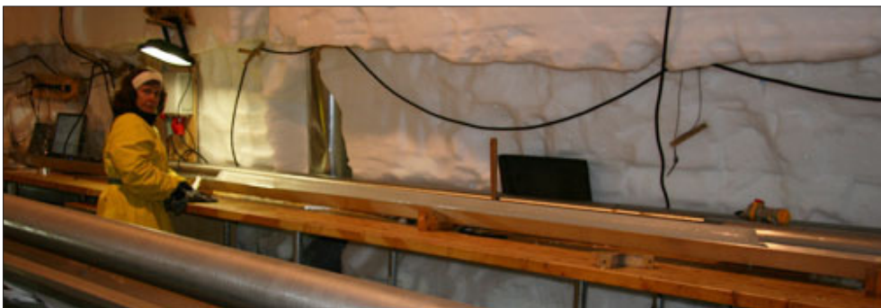
A 3.2 m long ice core from almost 2450 m depth is ready to be logged.
