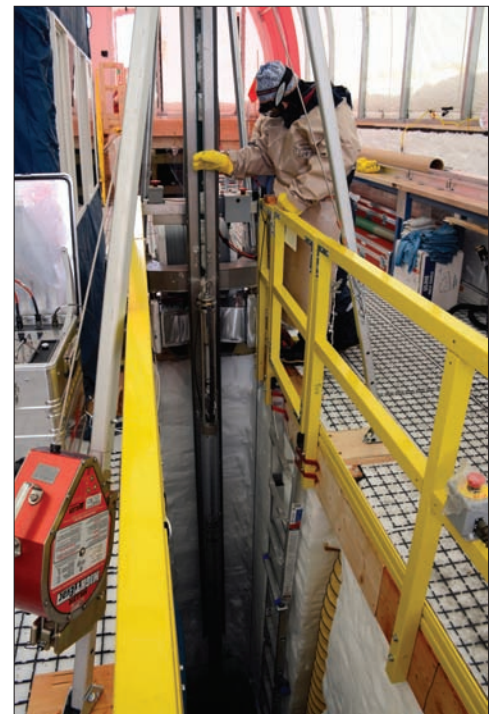
The drill returns to the surface after retrieving an ice core. —Credit: Peter Rejcek
