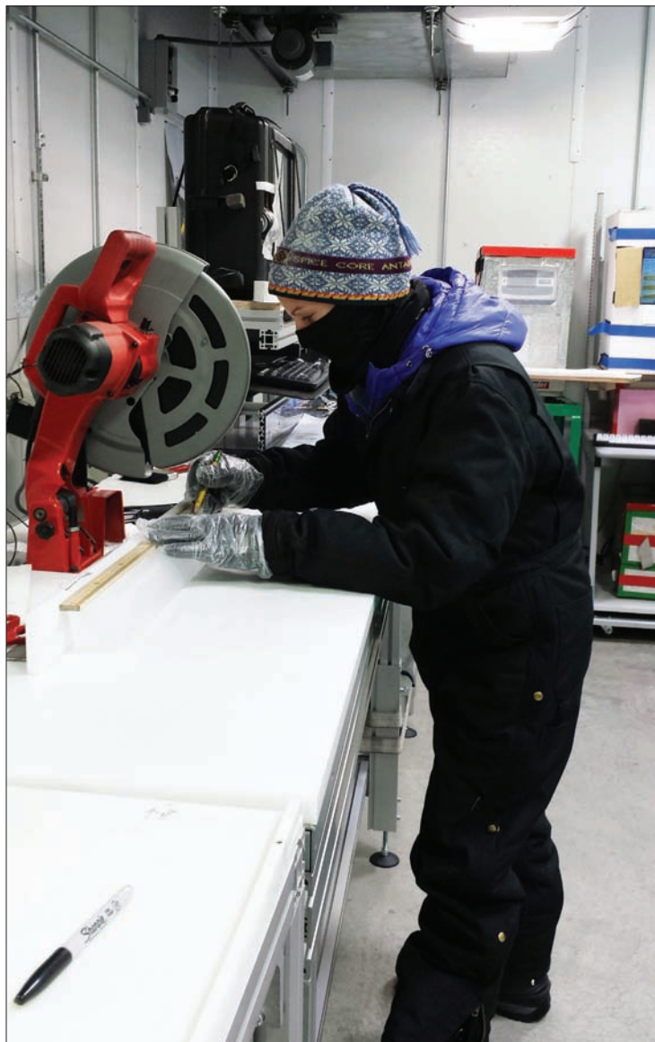
Mindy Nicewonger saws a section of an ice core that will be analyzed for its ancient trapped gases, such as carbonyl sulfide and ethane, during a core processing line at NICL. —Credit: Mindy Nicewonger
