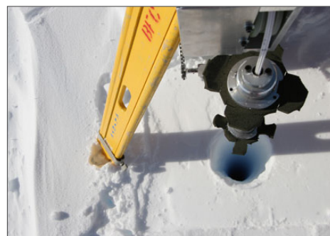
A view of the video camera before it is lowered into the borehole.
