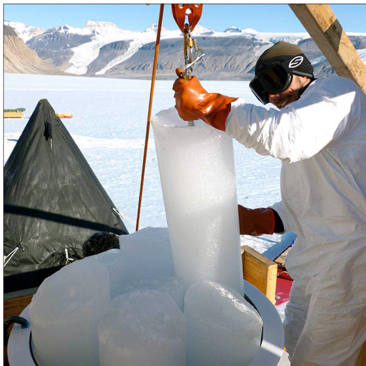
Vasilii Petrenko loading an ice core into the melting chamber for extraction of trapped ancient air. —Credit: Xavier Fain
