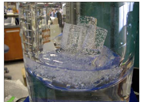
An ice core sample melts under vacuum to release the ancient air bubbles for isotopic analysis at a lab. Photo Credit: Anaïs Orsi
