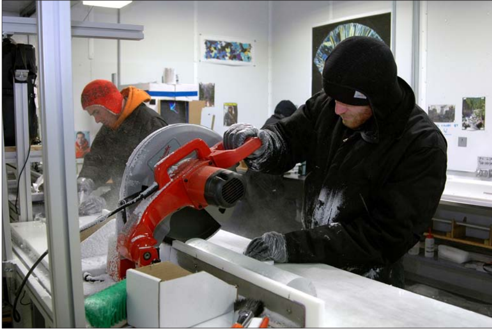
Logan Mitchell, from Oregon State University, saws a section of an ice core destined for gas measurements. The WAIS Divide researchers are particularly interested in measuring past concentrations of greenhouse gases like carbon dioxide and methane in the atmosphere. Photo Credit: Peter Rejcek
