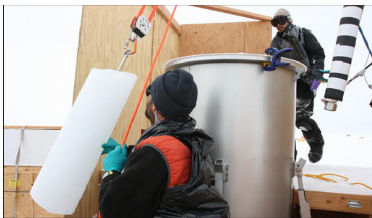
Drs. Hinrich Schaefer and Vasilii Petrenko load a one meter long section of core into the air extraction melter. Each core weighs about 40 kilograms. Photo Credit: Thomas Bauska
