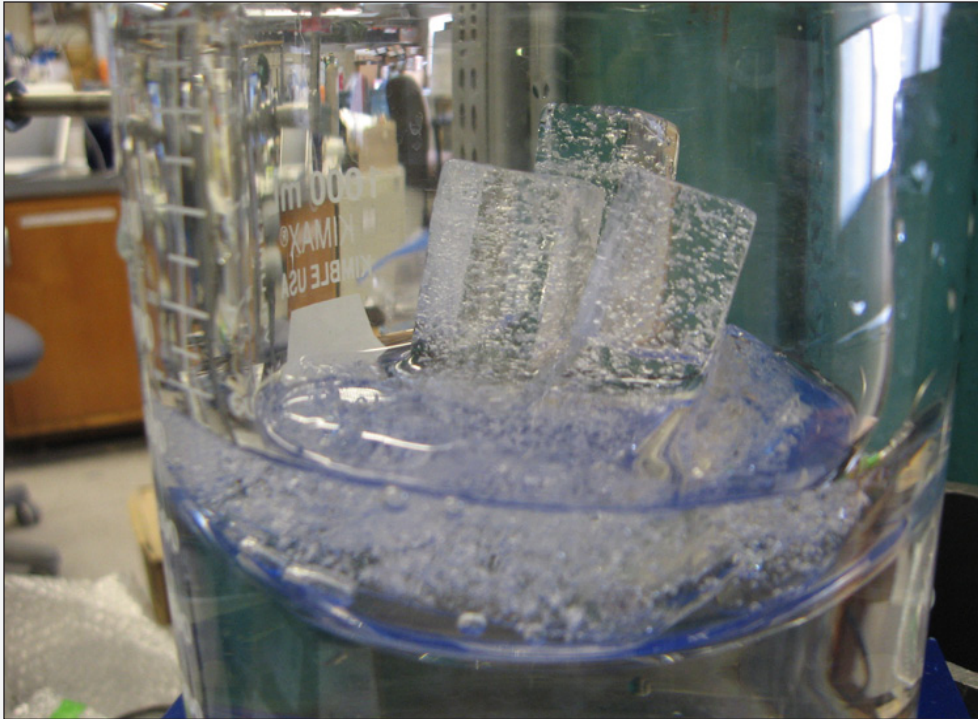
An ice core sample melts under vacuum to release the air bubbles. Photo courtesy of Anais Orsi, Scripps Institution of Oceanography.
