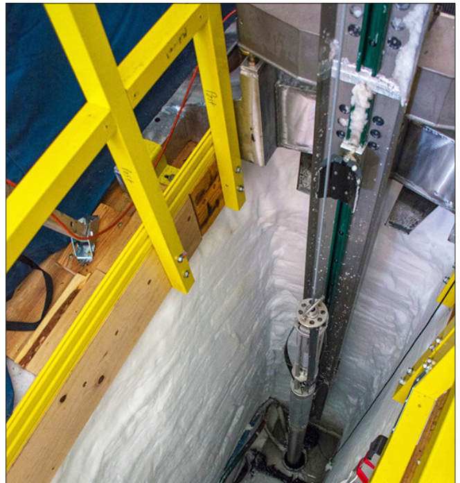
The SPICECORE drill hauls up an ice core from hundreds of feet below the surface. —Credit: Mike Lucibella
